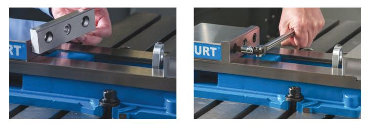
**Step 5** Install and tighten Sveconek Shaft (use 18mm open end wrench).
