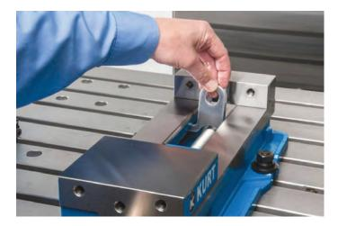
**Step 3** Secure Vise Movable Jaw against Vise Ways by tightening Movable Jaw adjustment screw. (Ref. Vise Manufacturers recommendation)
