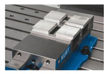
**Step 11** Clamp Sveconek Spacers as shown below between Sveconek Floating Jaw Plates to provide needed gap when machining Jaw Plates to hold your specifically shaped part.
