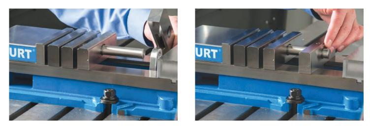
**Step 8** Bolt on Sveconek Fixed Jaw Plate. (with centered shaft clearance hole)
