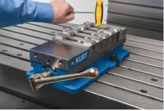
**Step 10** To remove parts from vise, first loosen Sveconek bracket set screw then loosen vise handle. \*\*Sveconek systems are completely versatile allowing you to hold various quantities of parts.\*\*
